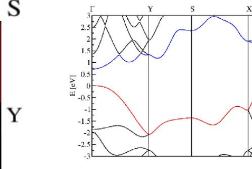
Electronic band structure of monolayer with direct band gap situtated at *Γ***-point** at **GGA PBE-D2** level.Red/blue solid line denotes Valence **BandMaxima/Conduntance** Band Minima (VBM/CBM).
